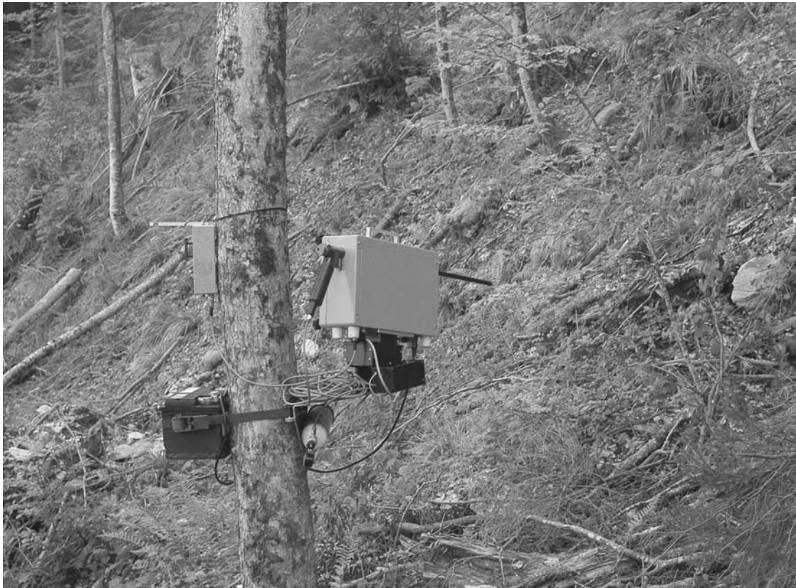
Figure 4. The minimally invasive capture system (MICS) mounted on a trunk platform 8 m from a dead chamois. Attached to the left side of the trunk are the battery and the antenna connecting the MICS with the control panel. The CO 2 tank is stored below the trunk platform.
